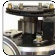
Precision magnetic pickup coil and reluctor.
